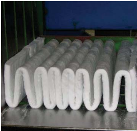
128kg/m 3 - 25mm thick SW607HT Blanket in folding process and final Z-Blok.
